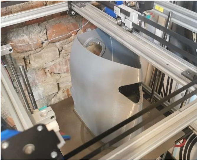
Fig. 3: Bow segment during 3D printing
